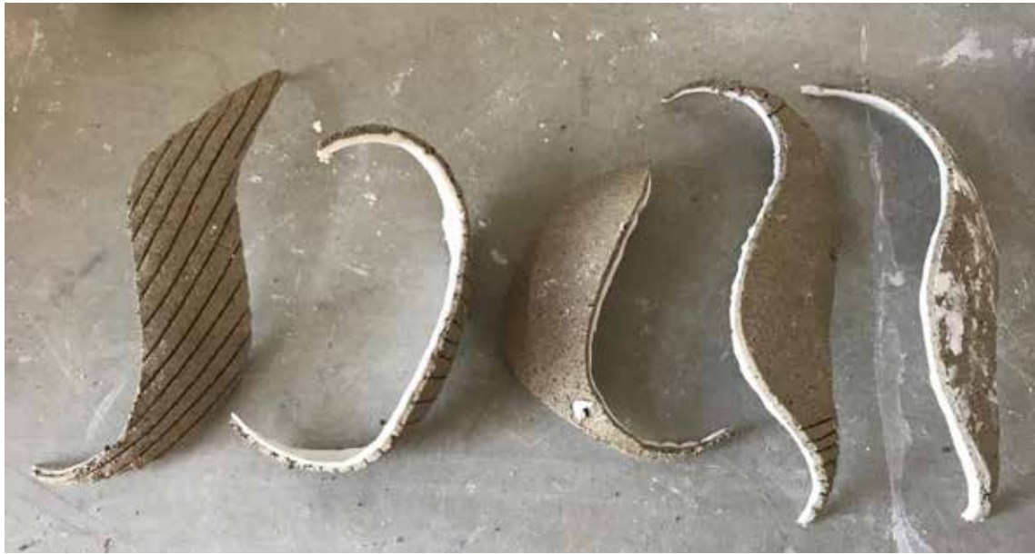
Figure 11. Oscillating curvature of two-dimensional contour curve creates significant displacement in resulting surface. Grooves on the terrazzo layer enable additional displacement and curvature.
